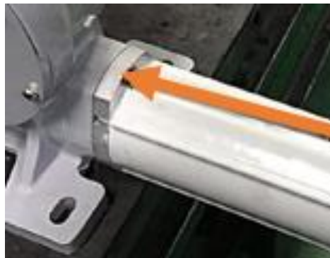
Fig. 11: Fitting DC motor.
