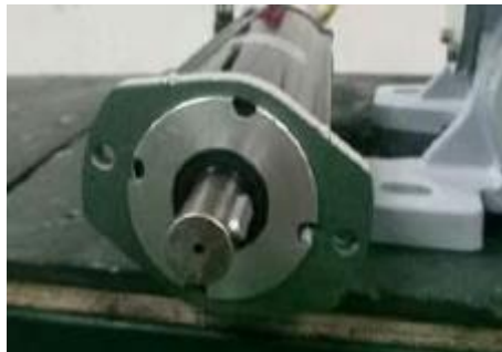
Fig. 8: Paper gasket fitting.
