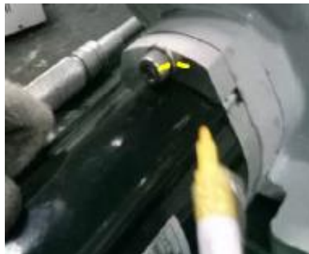
Fig. 15: Torque warning line.
