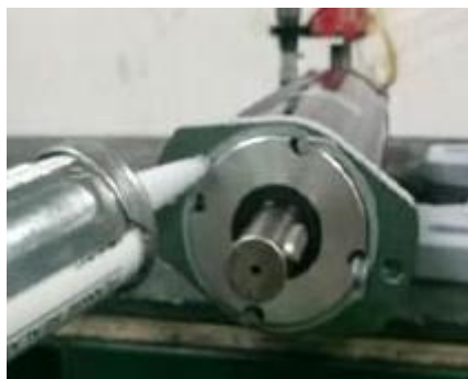
Fig. 9: Gasket sealant on the paper gasket.
